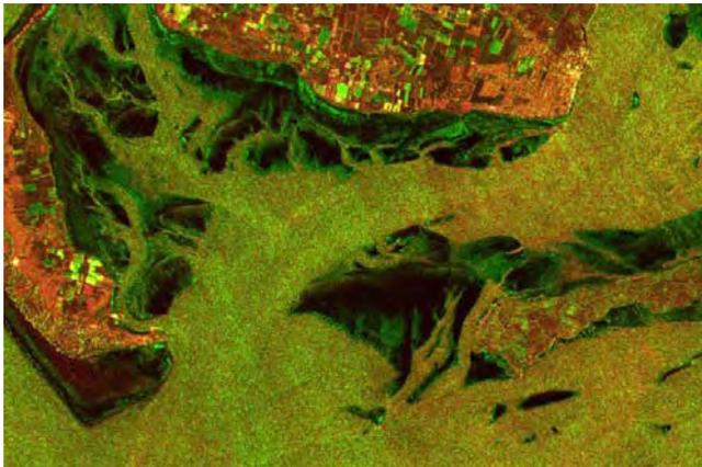
Figure 7. False-color composite of the two SAR images shown in Figure 6: ALOS PALSAR (red), ENVISAT ASAR (green), and their difference (blue).
