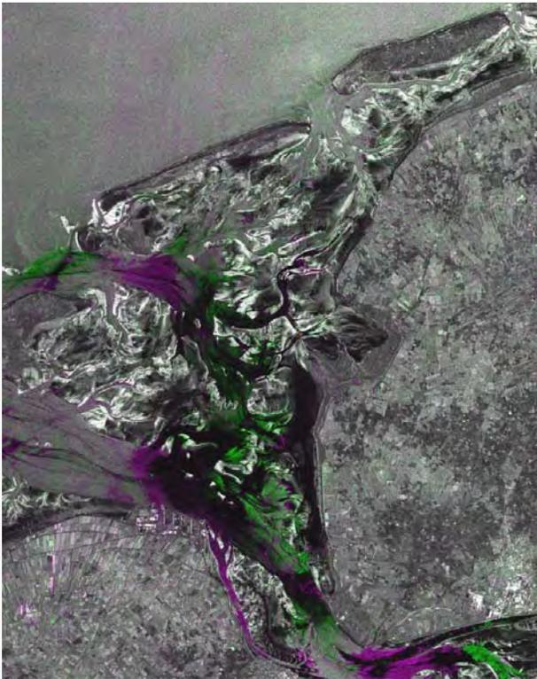
Figure 2. False-color composite of two SAR images (40 km × 50 km) acquired on July 27, 2008 over the river Ems estuary separating The Netherlands in the south-west and Germany in the north-east. Purple: ENVISAT SAR image acquired at 1001 UTC; green: ERS SAR image acquired at 1031 UTC. The bright patches in the image center are due to exposed intertidal flats south of the islands of Borkum (left), Juist (center), and Norderney (right).
