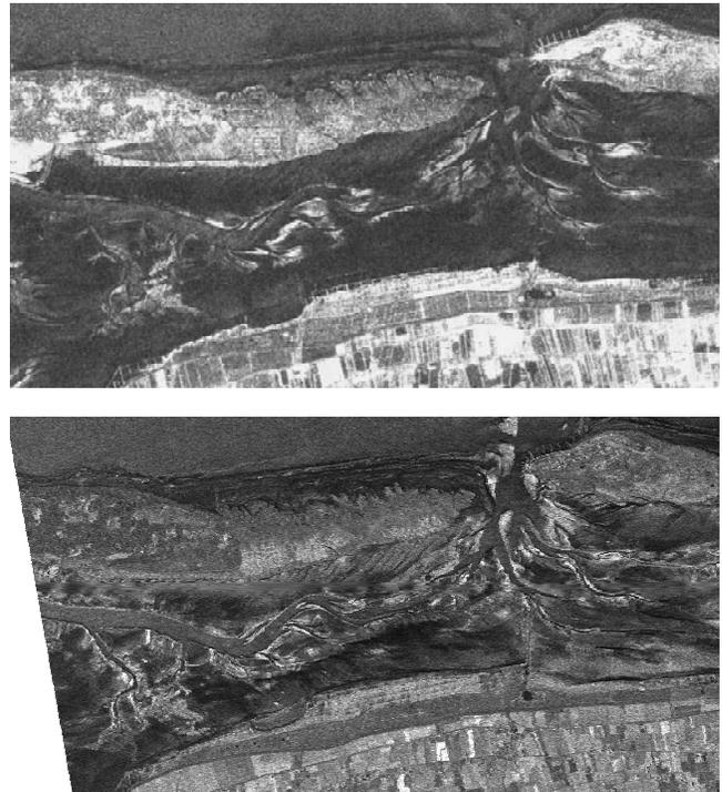
Figure 3. Two SAR images of the test site “Lütetsburger Plate”, south of the German island of Norderney (upper left part of the images), acquired shortly after low tide. Image dimensions are 25.7 km × 13.4 km. Top: ALOS PALSAR image (© JAXA 2008) acquired on April 12, 2008, at 2143 UTC; bottom: TerraSAR-X image (© DLR 2008) acquired on August 30, 2008, at 1710 UTC.
