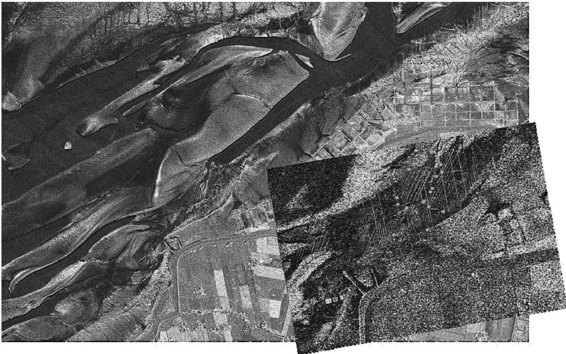
**Fig. 9:** Subsection of a TerraSAR-X image of intertidal flats north off the island of Pellworm in the “Halligenwatt” test area, acquired on 3 August 2009 (05:42 UTC, 54 minutes after low tide, 5-6 m/s wind from N).
