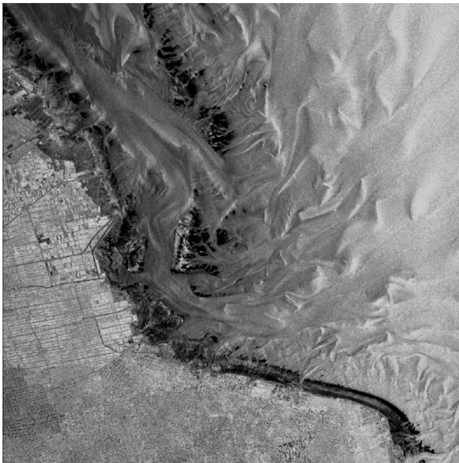
Fig. 7: ERS-1 SAR image ( 100 \text{ km} \times 100 \text{ km} ) of the Chinese Yellow Sea coast, north of the Yangtse estuary, acquired on July 8, 1995, at 02:34 UTC. Off the mainland coast signatures of underwater bottom topography and of dry-fallen intertidal flats can be seen as bright and dark features, respectively. (c) ESA 1995.
