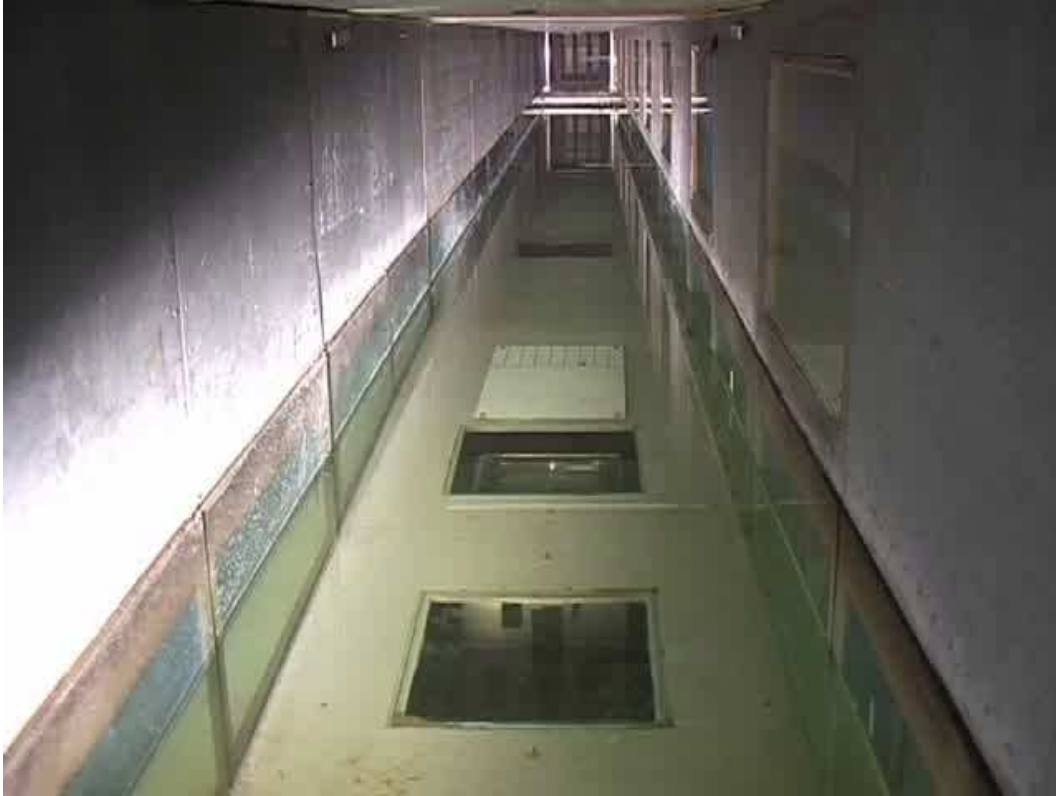
Fig. 3: photograph from inside the wind-wave tank. The quadratic windows at the tank's bottom are used for the laser wave-slope measurements.
