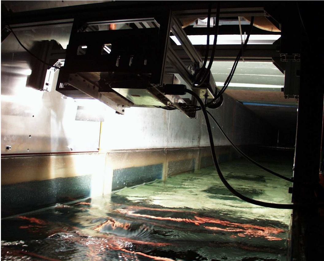
Fig. 5: photograph showing the upwind-looking W-band radar during a measurement with wind waves.
