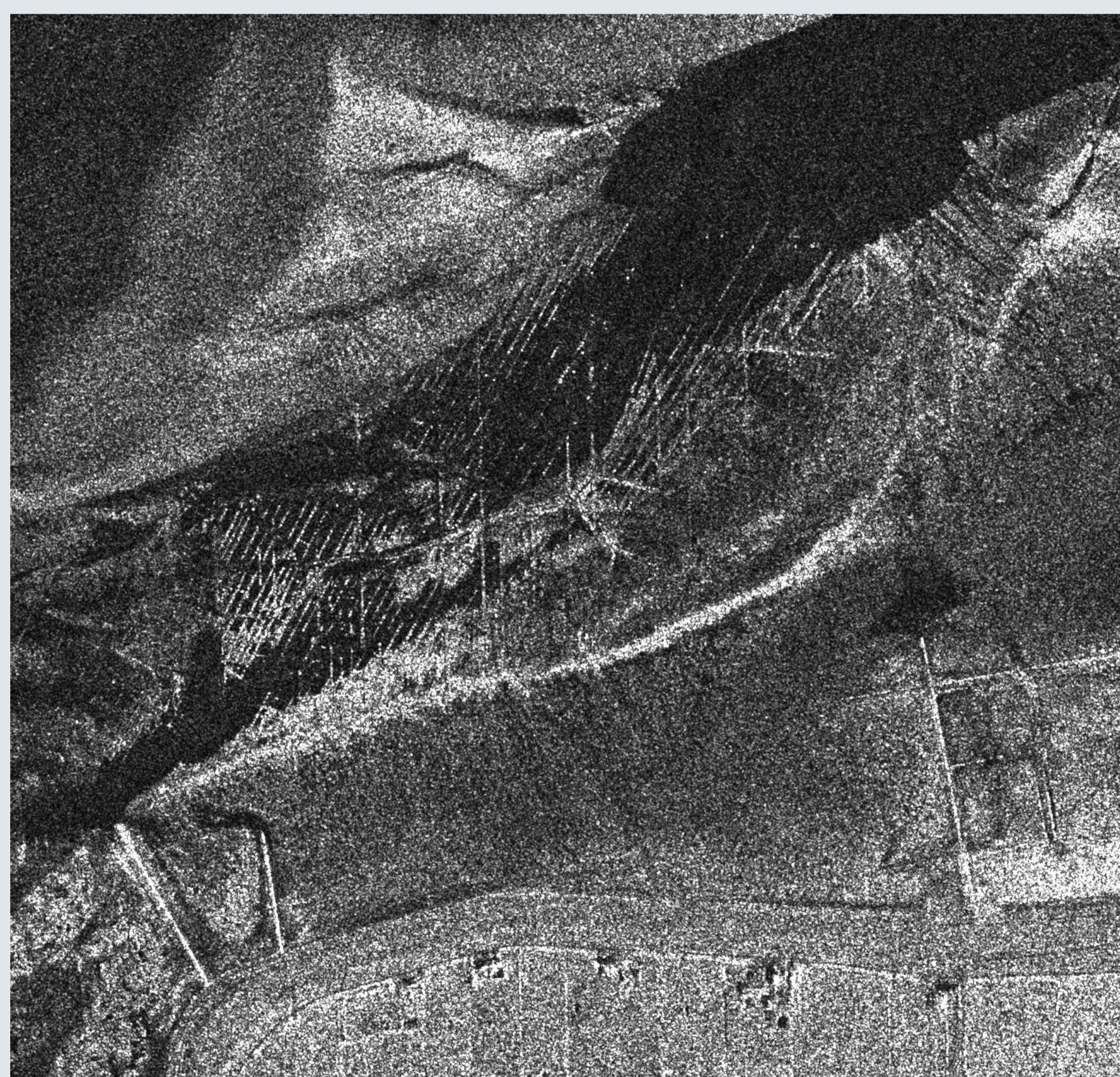
Section (1900 m × 2000 m) of a TerraSAR-X image of dry-fallen intertidal flats north of Pellworm. Residuals of historical land use can be delineated through linear bright and dark structures. © DLR 2009.
