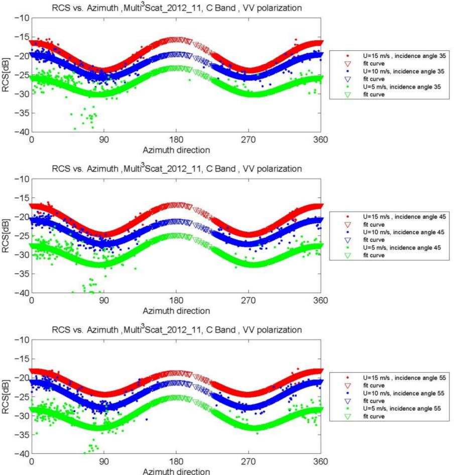
RCS versus azimuth angle for C band, vertical (VV) polarization, and wind speeds of 5 m/s (green),10 m/s (blue) and 15 m/s (red) at incidence angles  $35^{\circ}$ ,  $45^{\circ}$ ,  $55^{\circ}$  (top to bottom). Added are fits to the data according to the GMF presented above.
