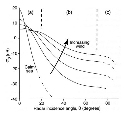
Normalized Radar Cross Section,  $\sigma_0$ , as a function of incidence angle, and its change with increasing wind speed (Robinson 2004). The regions (a), (b) and (c) indicate different dominant scattering mechanisms. Multi<sup>3</sup>Scat measurements were performed only in region (b) (Bragg scattering).
