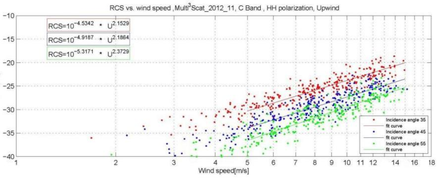
Wind-dependent RCS at C band, vertical (VV, upper panel) and horizontal (HH, lower panel) polarization, for incidence angles  $35^{\circ}$  (red),  $45^{\circ}$  (blue) and  $55^{\circ}$  (green). Shown are all upwind measurements in November 2012.
